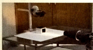
Fig. 1: Imaging with front light source (for illumination of sample)
